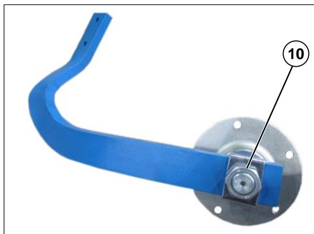
The nuts (10) on the front and rear rows of hollow discs have different threads.
