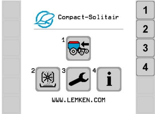
The Main menu appears after switching on the electronic control system and a brief system check.
