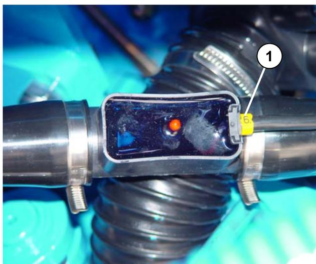
Each seed flow sensor on the implement has been assigned a number (1).
