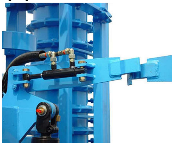
Hydraulic transport lock for the lateral sections
