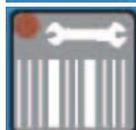
Rhythm key for the automatic determination of the tramline rhythm after entering the working width of the following implement
