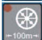
Calibration key for the 100 m calibration in cm per pulse
