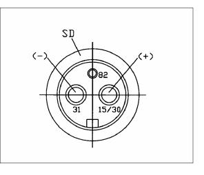
Excess-voltage and undervoltage can lead to malfunctions and probably can destroy the electronic components. Furthermore a fuse protection of the power supply of at least 25 A must be ensured.
