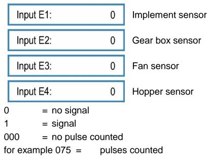
The sensors E1 to E3 give a signal, when they have contact to a metallic thing (distance apprs. 2 mm). The sensor E4 (hopper sensor) gives a signal, when there is no contact to seed.
