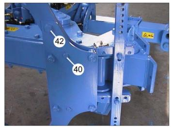
All Euro-Titan and Euro-Titan X ploughs are fitted with shearbolts (40) as standard.
