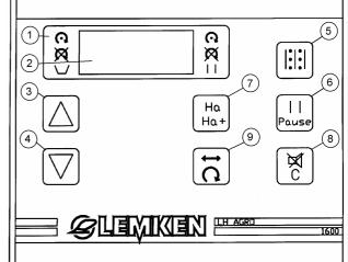
5 Operation-key for adjusting the tramline rhythm, operating position
