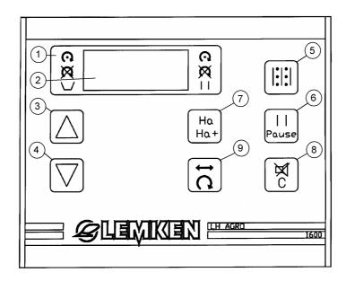
Before entering the wheel circumference in cm per impulse the clear-key (8) has to be pressed shortly to set the indicated value to zero.
