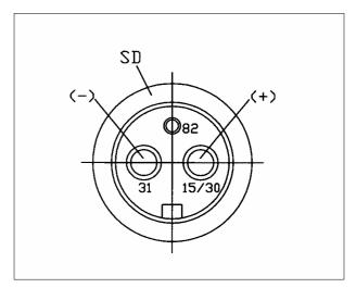
fuse of the socket (SD) and then the fuse (SI) at the circuit box between plug and on-board computer. If the fuses are not blown, the polarity of the socket (SD) must be reversed.
