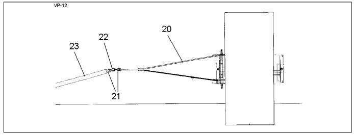
The VarioPack can also be used in combination with semi-mounted conventional ploughs in conjunction with a drawbar (20).
