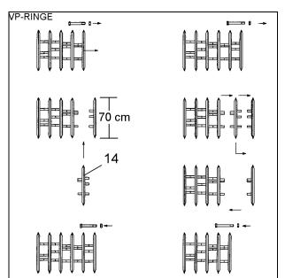
If possible, the same number of packer rings should be bolted to the left and right of the frame.
