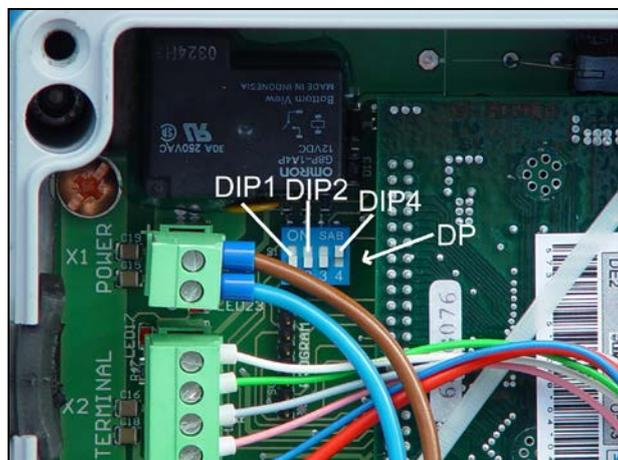
Depending on the working width and the type of implement, the seed drill control has been adjusted correspondingly in the factory. Therefore the DIP-switches (DP) have been set to ON or OFF – see section “Adjustment of the DIP-switch”.
