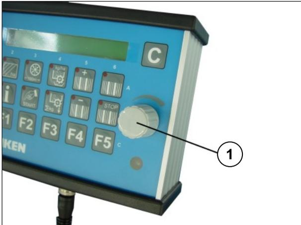
Values and adjustments will be chosen by means of the rotary switch (1). Therefore the head of the rotary switch must be turned correspondingly. The following part of the operation instructions speaks about “choosing” and “encoding”. That means always the operation of the rotary switch.
