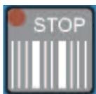
Stop key for activating and deactivating the tramline mechanism
