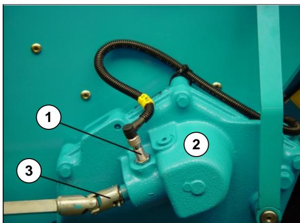
For measuring the distance, the pulses will be counted by means of the sensor (1). These pulses will be generated by a pulse pickup in the gear box (2).
