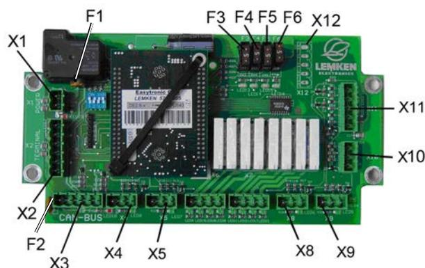
The circuit board with the connector sockets, fuses and LEDs is located in the distributor box.
