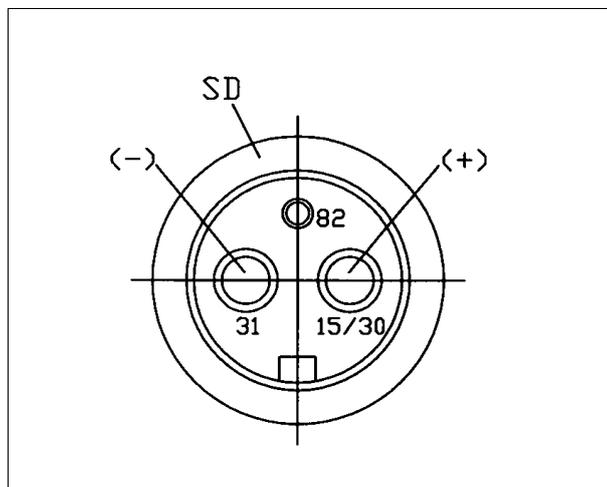
For the power supply of the electronic seed drill control a socket according to DIN 9680 must be provided at the tractor.
