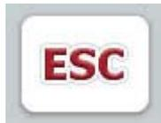
By using the "ESC" button, the input is aborted in all input dialogues. The previous value is maintained.
