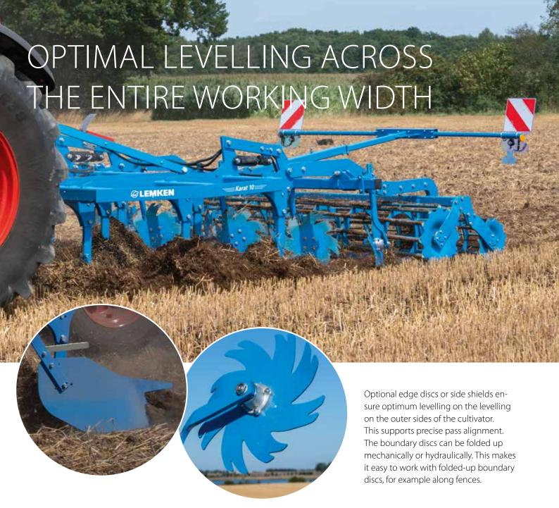
Centrally adjustable levelling elements provided behind the tine section ensure even levelling. Specially shaped star wheels are optionally available, which run ahead of the roller for optimal results, particularly in heavy soils.
