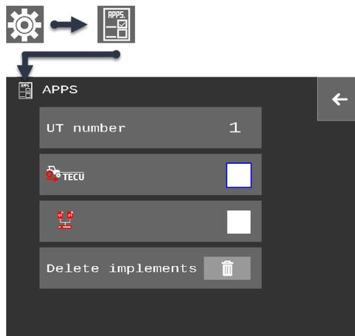
► On an ISOBUS tractor, switch off the CCI 60 TECU in the "App Settings".
