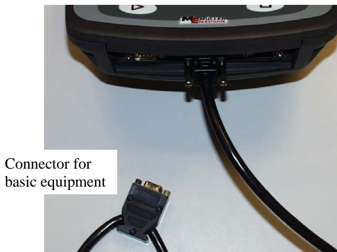
Diagr. 3-9 BASIC - Terminal with MFG connecting cable and connection for the basic equipment
