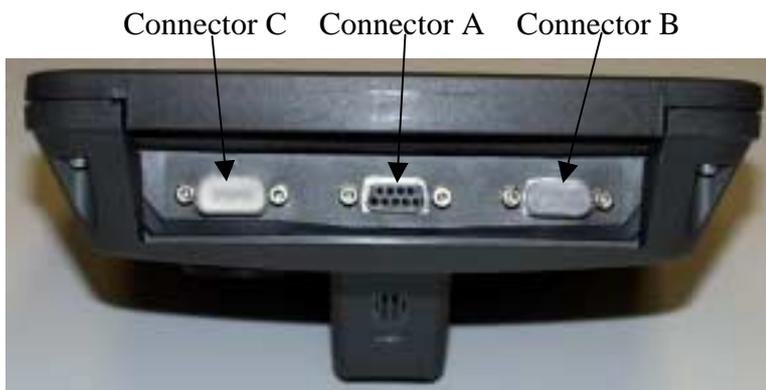
Diagr. 3-7 Connections at the bottom of the *BASIC - Terminal*
