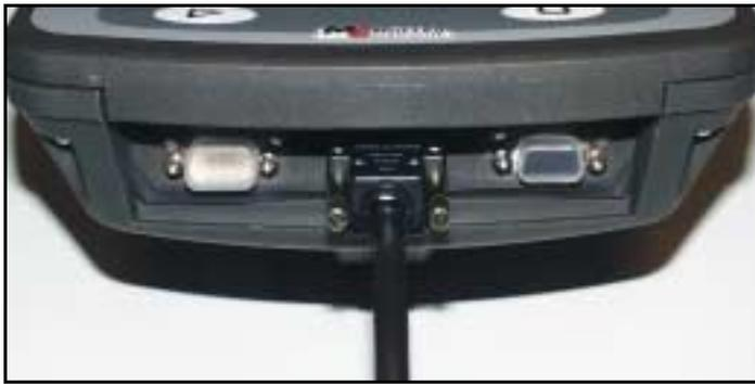
Diagr. 3-8 BASIC - Terminal with connecting cables from the basic equipment
