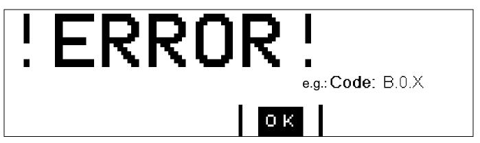
The failure message will be confirmed by pressing the OK-button. The horn stops and the failure message disappears on the display. Only the shining of the light-emitting diodes shows that there is still a malfunction.
