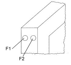
The fuse F1 is a slow glass fuse with 1 A (part No.: 373 1306) and the fuse F2 is a slow glass fuse with 16 A (part No.: 373 1308).
