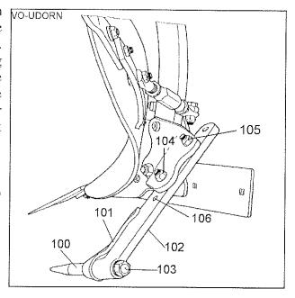
Never use bore (106) as this will cause the loss of the subsoiler if the bolt (104) shears!
