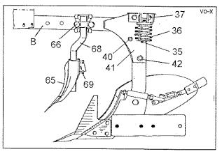
Only the rear bores with the beam (B) may be used as the front bores are reserved for disc coulters. Tighten nut (66) carefully after adjustment.
