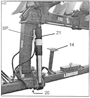
For transport the plough frame must be turned in halfturned position! After that the lock valves (SP) of both rams (21) must be locked!
