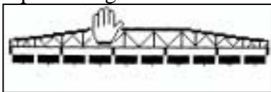
**Diagram 4-18 Boom sections; main switch off; all sections are pre-selected**
