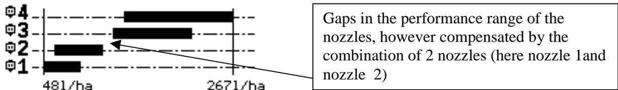
On the other hand the performance range diagram may not display gaps, however combining nozzles over the whole range is not entirely possible. This occurs in particular in connection with tandem fittings.
