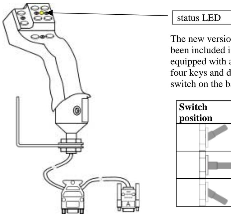
The new version of the multifunction grip has been included in delivery since May 2004. It is equipped with a LED status between the top four keys and displays the current status of the switch on the back of the multifunction grip.
