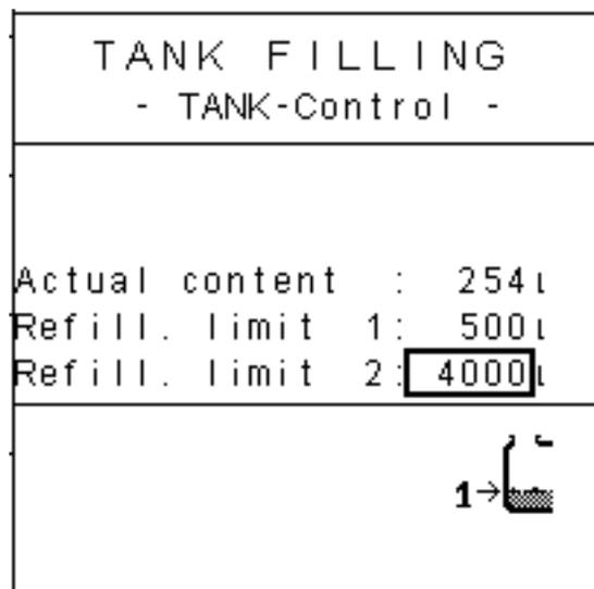
Diagram 4-29 Filling with 2 filling limits
