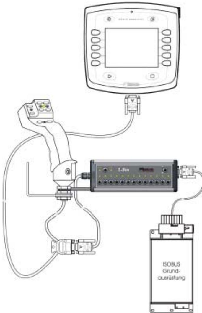
**Diagram 12-3 Wiring with MFG**
