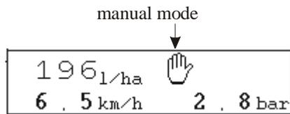
**Diagram 4-15 Manual spraying mode**
