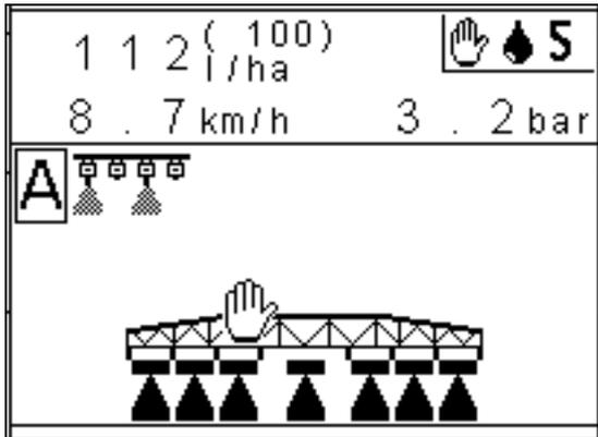
Diagram 10-3 Illustration of multiple nozzles in the working mask
