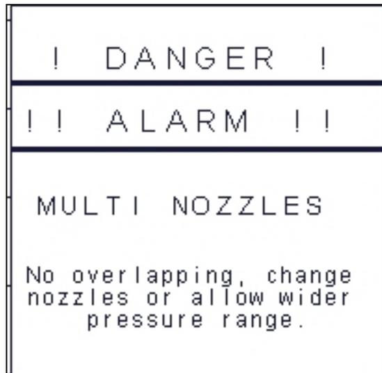
In order to get a better understanding for the reason behind the alarm, refer to the diagram illustrating the performance range of the nozzles and press the
