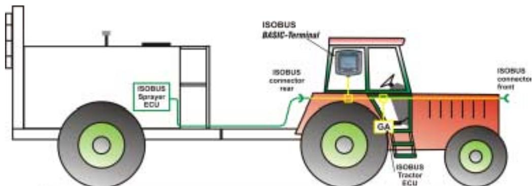
**Diagram 1-1 Basic configuration of the ISOBUS according to ISO Standard 11783**
