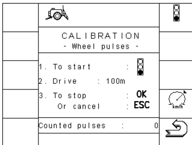
Diagram 4-9 Calibration of wheel sensor
