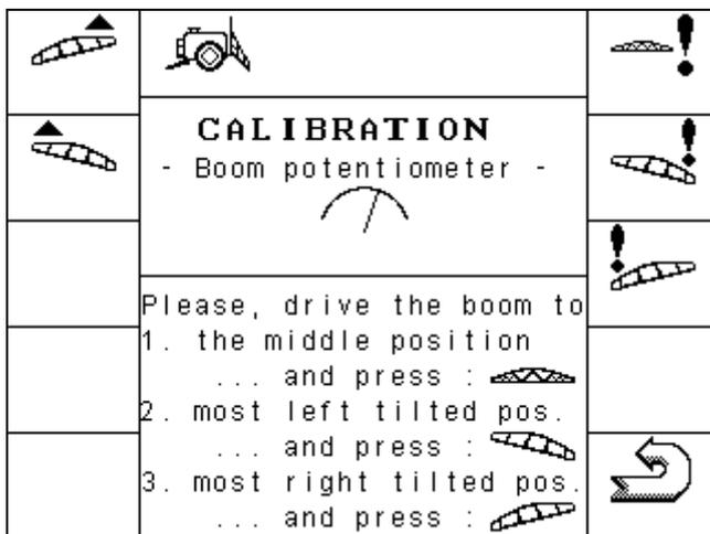
Diagram 5-1 Calibration slope levelling
