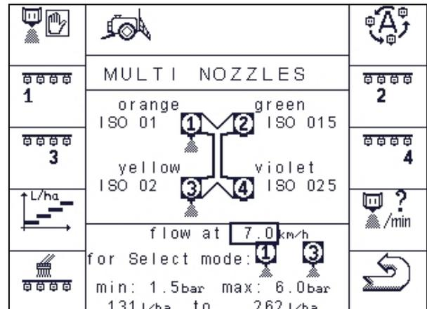
Diagram 10-5 Multiple nozzles mask in Select mode
