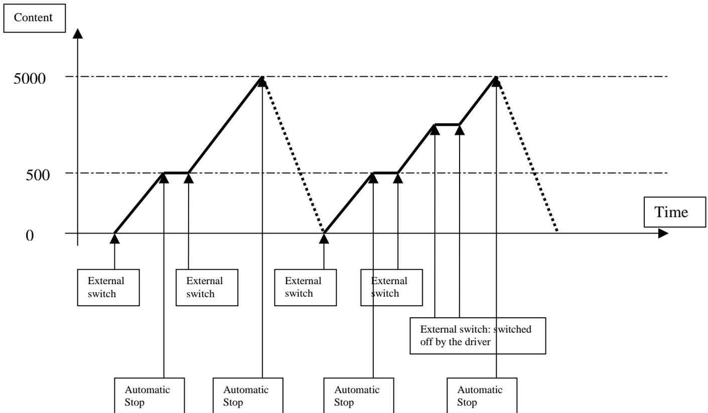
As the diagram illustrates, the filling process can be interrupted using the external switch without altering the sequence of the 2-stage filling.
