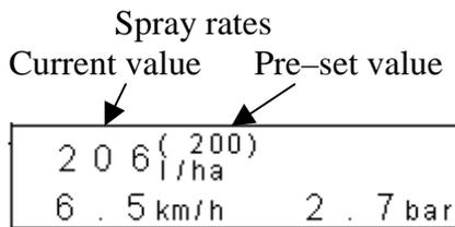
Diagram 4-13 Spraying data in the working mask
